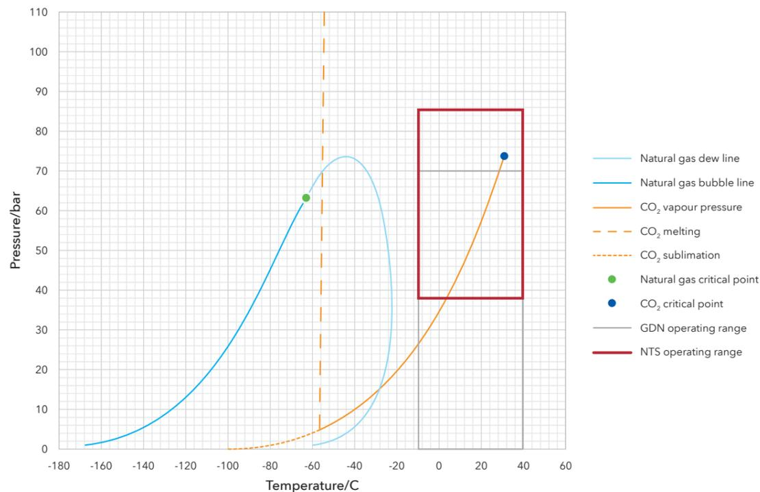
Figure 1: Comparison of the phase envelopes of natural gas and CO<sub>2</sub>
