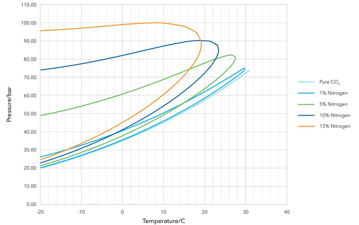
Figure 2: Phase behaviour of CO<sub>2</sub> + N<sub>2</sub> mixtures
